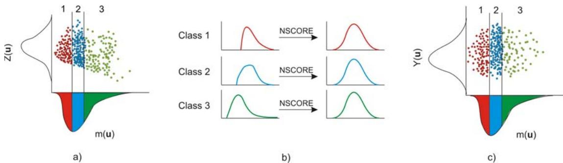
Fig. 1 Schematic illustration of the stepwise conditional transform with the trend model as the primary variable,  $m(\mathbf{u})$ : (a) partition the original variable,  $Z(\mathbf{u})$  into probability classes, (b) subset the secondary data into conditional distributions and normal score transform each class independently, and (c) the resulting transform yields a transformed secondary variable,  $Y(\mathbf{u})$ , that is both Gaussian and uncorrelated to the trend.
